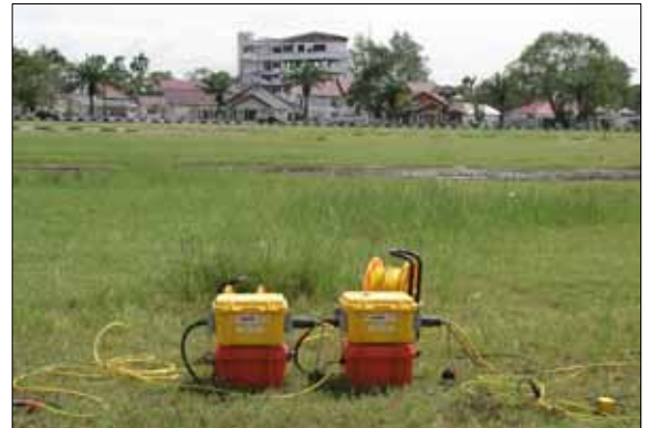
Fig. 2: Shallow shear wave site investigation at Plang Padang place, centre of Banda Aceh city. Foreground: 48 channel Geode system used for seismic data acquisition. Middle: Local mud zone indicating local subsidence of young sediments. Background: Small houses of nearly traditional Indonesian building style are only minor affected by earthquake shakings. By contrast, the high concrete building shows heavy structural damages up to total collapse due to the earthquake shakings of 26th Dec. 2004.
