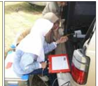
Fig. 2: Shallow shear wave site investigation at Plang Padang place, centre of Banda Aceh city. Foreground: 48 channel Geode system used for seismic data acquisition. Middle: Local mud zone indicating local subsidence of young sediments. Background: Small houses of nearly traditional Indonesian building style are only minor affected by earthquake shakings. By contrast, the high concrete building shows heavy structural damages up to total collapse due to the earthquake shakings of 26th Dec. 2004.
