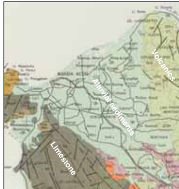
Fig. 1: Cut out of the official geologic map (1981) of the Krueng Aceh river delta showing undifferentiated alluvial sediments of holocene age for the whole investigation area. Post tsunami groundwater exploration drillings yield stacks of organic clay, silt, sand and gravel down to a depth of 220 m without any hints of the basement contact.
