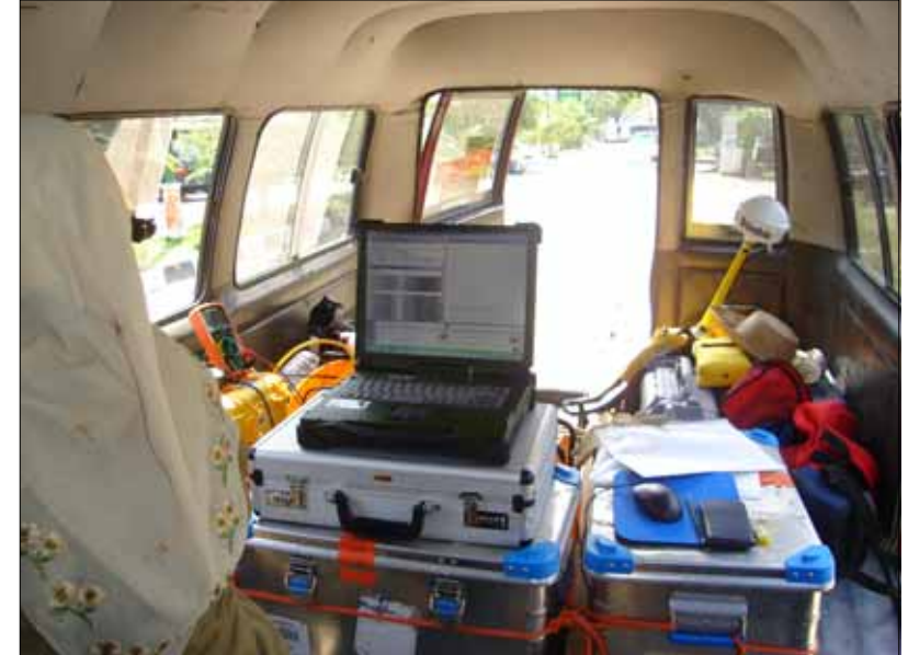
Fig. 2: Operators seat inside the recording van with 48 channel Geode recording system installed (stack of yellow boxes at left). The whole equipment including spare parts could be integrated into the hired van. Differential GPS (background right) has been used for positioning.
