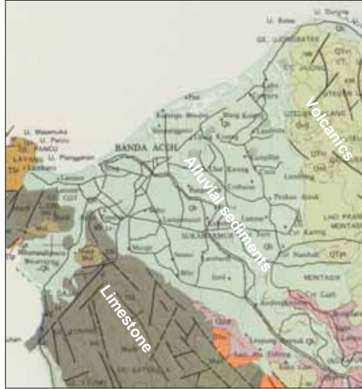
Fig. 1: Detail of the official geologic map (1981) of the Krueng Aceh river delta showing undifferentiated alluvial sediments of holocene age for the whole investigation area. Post tsunami groundwater exploration drillings yield stacks of organic clay, silt, sand, and gravel down to a depth of 220 m without any hints of the basement contact.
