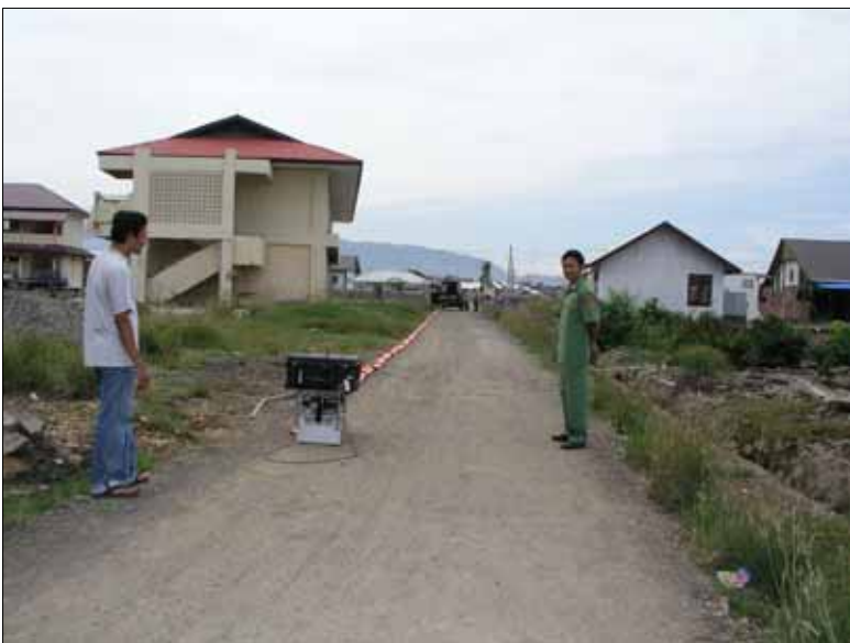
Fig. 3: Investigation site Kampong Jawa (A) in the floodplain area near the coast line now in preparation for reconstruction. The land streamer has been positioned at the left side of the dirt road to enable traffic bypass.
