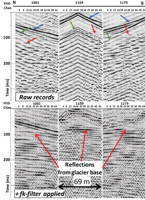
Fig. 5: During processing of Colle Gnifetti data, fk-filtering was the most important process to attenuate Love surface waves (green arrows) and direct arrivals (blue, ~1400 m/s). Only some weak reflection events (red arrows) could be observed in the raw data prior to fk-filtering, whereas clear basement reflections are visible after filter application.
