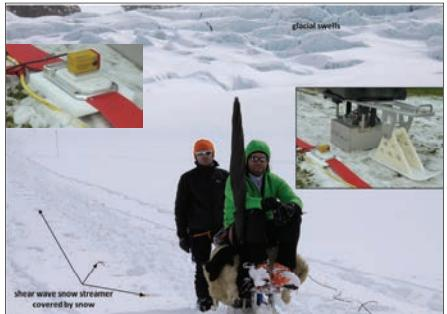
Fig. 3: ELVIS horizontal vibrator source in operation on Gepatschferner profile 1. The land streamer is almost covered by fresh fallen snow.
