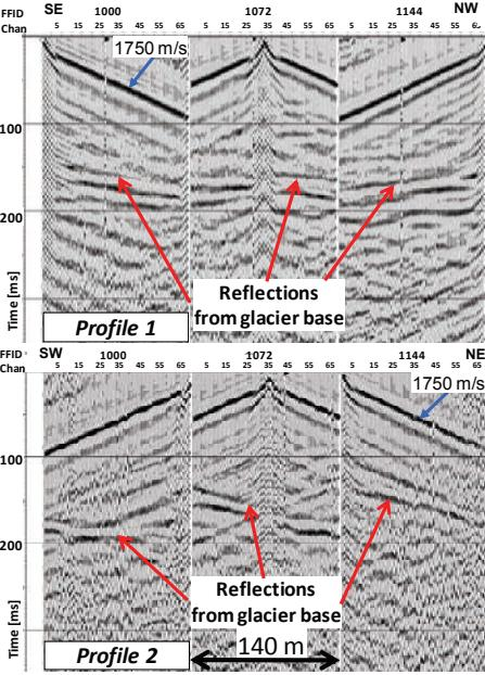
Fig. 6: During processing of Gepatschferner data, fk-filtering was of less importance. Reflections from the basement below the ice could be clearly detected in the raw records. Probably due to the fresh fallen snow at the surface, frequency content of the data was lower compared to the Colle Gnifetti data.
