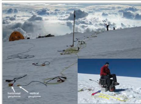
Fig. 2: Impression from the seismic survey setup above the clouds in an altitude of about 4500 m a.s.l. at Colle Gnifetti. Vertical (for an additional P-wave survey) and horizontal geophones were planted simply at the snow surface.
