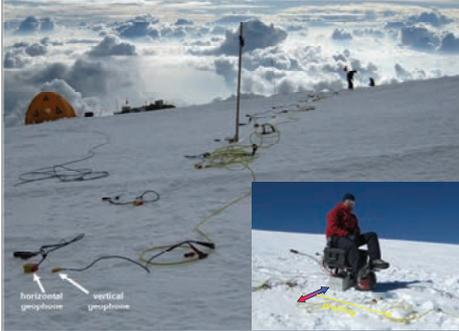
Fig. 2: Impression from the seismic survey setup above the clouds in an altitude of about 4500 m a.s.l. at Colle Gnifetti. Vertical (for an additional P-wave survey) and horizontal geophones were planted simply at the snow surface.
