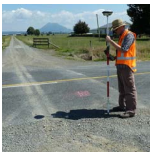
Fig. 9: Profiling positions painted on the roads during data acquisition were subsequently recorded by LEICA DGPS positioning in high-resolution. In the background: Mount Edgecumbe, the dominating volcano in the area.
