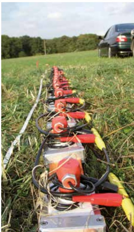
In operation with geophones at 25 cm intervals
